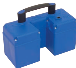
Quick-change battery unit BU PT 5,2 Ah weight 4.3 kg, capacity 5.2 Ah, voltage 24 VDC Art. No. 004 150
